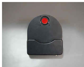
CFW10 Color Filter Wheel with ten filter positions for 1.25" filters
